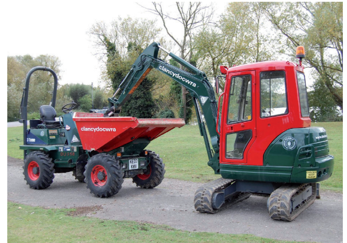
Secure equipment together preventing either being lifted or dragged away. Use immobilisers and/or hydraulic locks with chain and padlocks.
