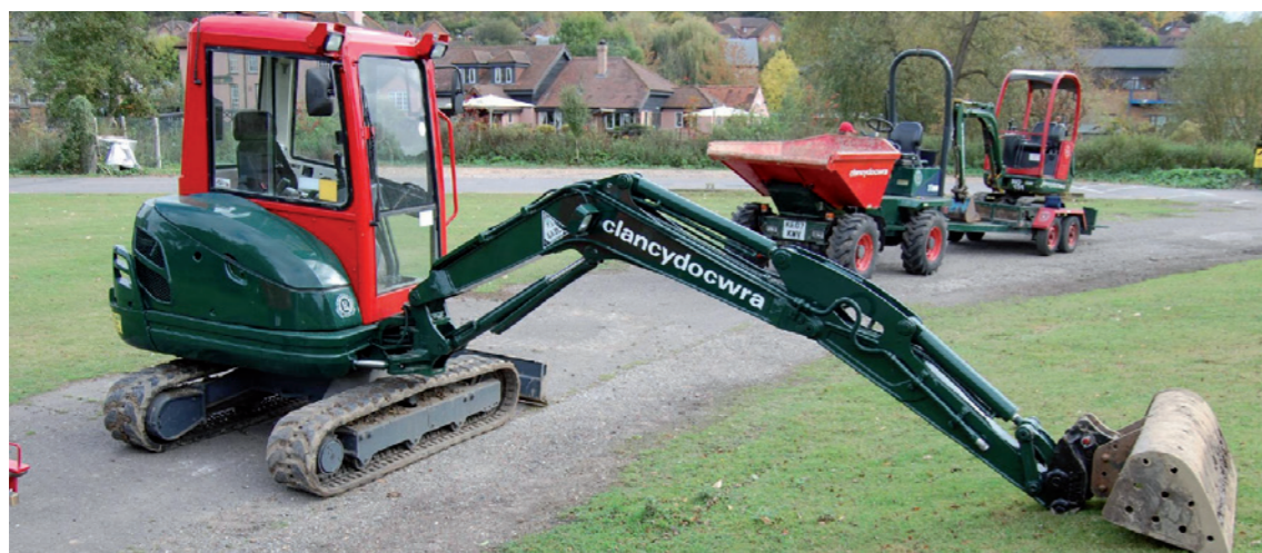
If leaving mini excavators remove from trailer, slew cab and extend boom arms. Use immobilisers and/or hydraulic locks. This makes the machine impossible to remove or lift away. Note the use of CESAR registration and corporate livery. Criminals dislike stealing this type of equipment due to expense of repainting equipment.
