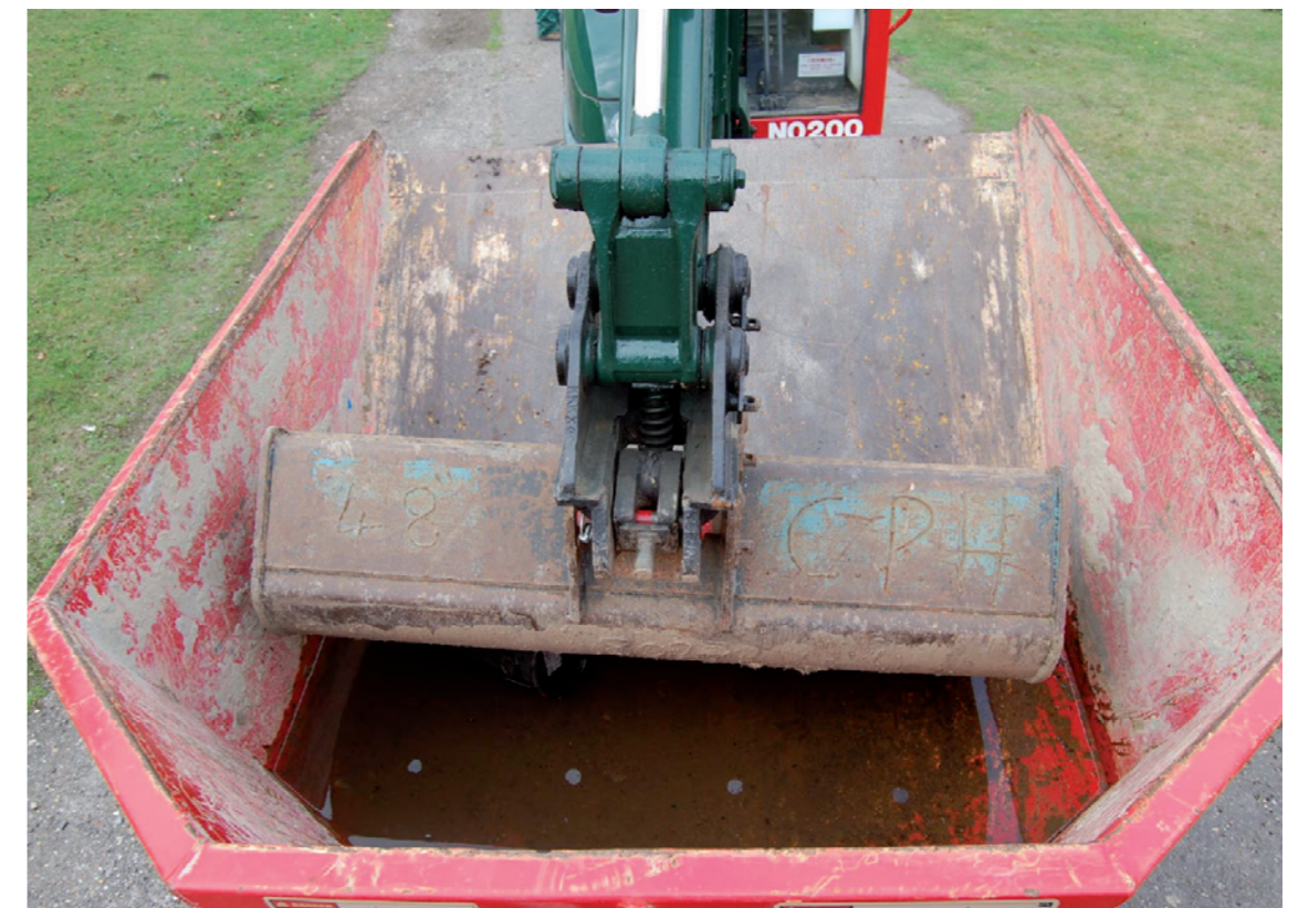
For attachments and buckets weld plant numbers and company logos/details to aid identification.
