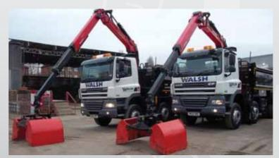
Each fitted with PALFINDER Hydraulic grab Buckets Image above is of RK12YBT and RK12YBS
