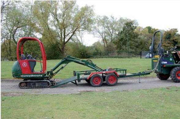
*Make the thief's life harder. Equipment removed from trailer and boom arms extended and immobilisers and/or hydraulic locks set preventing ease of theft.*
