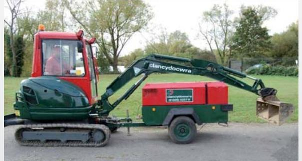
When leaving equipment overnight on sites secure compressors under boom arms of mini excavators then use immobilisers or hydraulic locks to prevent removal.
