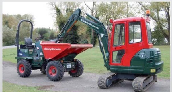
Secure equipment together preventing either being lifted or dragged away. Use immobilisers and/or hydraulic locks with chain and padlocks.
